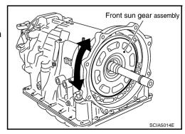
51. Install needle bearing to front sun gear.
