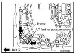
Connect A/T fluid temperature sensor 2 connector.
