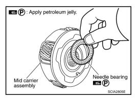
45. Install mid carrier assembly in rear carrier assembly.
