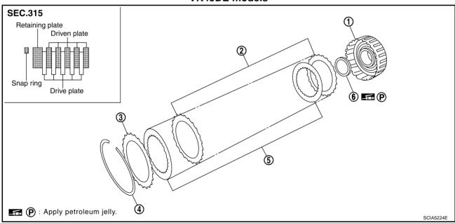
High and low reverse clutch drum
