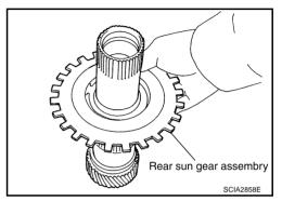
a. Using a flat-bladed screwdriver, remove snap ring from rear sun gear.
