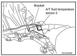
Install A/T fluid temperature sensor 2 (with bracket) in control valve with TCM, and then tighten A/T fluid temperature sensor 2 mounting bolt to the specified torque. Refer to <u>AT-239, "COM-PONENTS"</u>.
