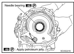
72. Remove parking actuator support from rear extension (2WD models) or adapter case (AWD models).
