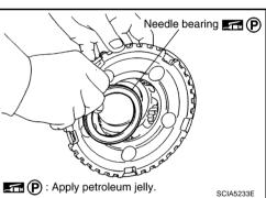
c. Remove snap ring from front carrier assembly.
