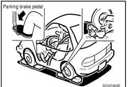
6. Start the engine, then measure the line pressure at both idle and the stall speed.
