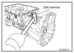
iii. Remove adapter case assembly from transmission case. (With needle bearing)
