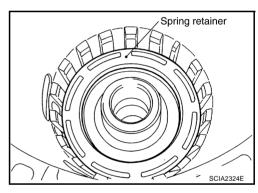
17. Set the SST on spring retainer and install snap ring (fixing spring retainer) in transmission case while compressing return spring.
