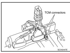
41. Remove A/T assembly harness connector from control valve with TCM using a flat-bladed screwdriver.
