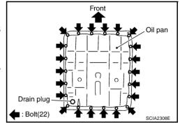
c. Tighten oil pan mounting bolts to the specified torque in numerical order shown in the figure after temporarily tightening them. Refer to <u>AT-239</u>, "COMPONENTS".
