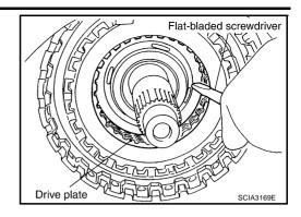
39. Install high and low reverse clutch hub, mid sun gear assembly and rear sun gear assembly as a unit.
