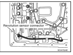
14. Straighten terminal clip to free revolution sensor harness.
