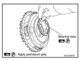
b. Remove needle bearing from front carrier assembly. (VK45DE models)
