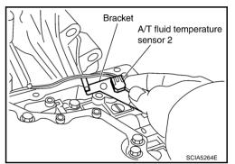
2. Install A/T fluid temperature sensor 2 (with bracket) in control valve with TCM, and then tighten A/T fluid temperature sensor 2 mounting bolt to the specified torque. Refer to AT-239, "COM-PONENTS".
