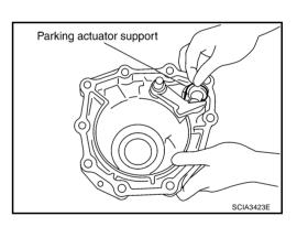
17. Remove parking pawl (with return spring) and pawl shaft from rear extension.
