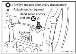
49. Install brake band in transmission case.
