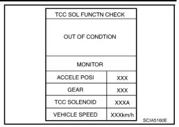
When testing conditions are satisfied, CONSULT-II screen changes from "OUT OF CONDITION" to "TESTING".
