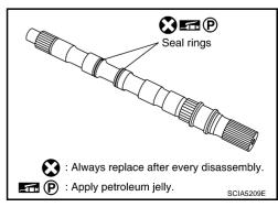
31. Install parking gear to output shaft.
