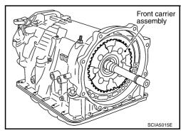
14. Loosen lock nut and remove band servo anchor end pin from transmission case.
