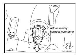
15. Install snap ring to A/T assembly harness connector.
