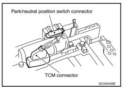
2. Install A/T assembly harness connector from control valve with TCM.
