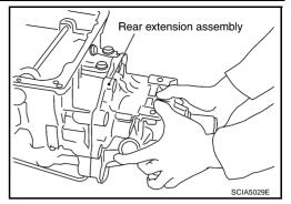
iii. Tighten rear extension assembly mounting bolts to specified torque. Refer to <u>AT-274, "Components"</u>.
