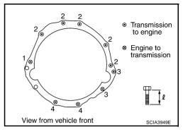
Align the positions of tightening bolts for drive plate with those of the torque converter, and temporarily tighten the bolts. Then, tighten the bolts with the specified torque. Refer to <u>AT-266</u>, <u>"COMPONENTS"</u>.
