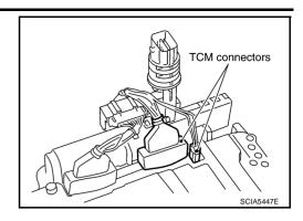
4. Install O-ring in A/T assembly harness connector.
