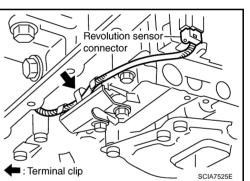
16. Remove revolution sensor from transmission case.
