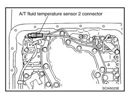
Securely fasten A/T fluid temperature sensor 2 harness with terminal clip.
