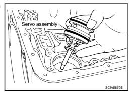
69. Remove return spring from servo assembly.
