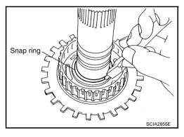
3. Remove high and low reverse clutch hub from mid sun gear assembly.
