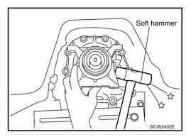
10. Remove rear extension assembly from transmission case. (With needle bearing.)
