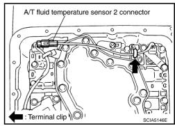
Remove A/T fluid temperature sensor 2 with bracket from control valve with TCM.
