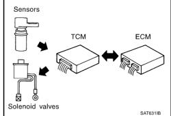
It is much more difficult to diagnose a error that occurs intermittently rather than continuously. Most intermittent errors are caused by poor electric connections or improper wiring. In this case, careful checking of suspected circuits may help prevent the replacement of good parts.
