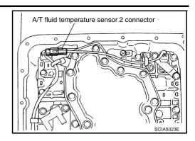
11. Securely fasten terminal cord assembly and A/T fluid temperature sensor 2 harness with terminal clips.
