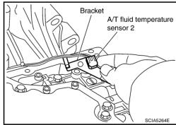
f. Install A/T fluid temperature sensor 2 (with bracket) in control valve with TCM, and then tighten A/T fluid temperature sensor 2 mounting bolts to the specified torque. Refer to <u>AT-274, "Components"</u>.
