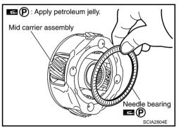
44. Install needle bearing (front side) to mid carrier assembly.
