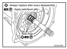
13. Remove front carrier assembly from rear carrier assembly. (With input clutch assembly and rear internal gear.)
