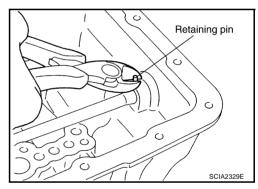
62. Remove manual plate (with parking rod) from manual shaft.
