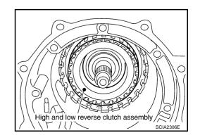
38. Using a flat-bladed screwdriver, align drive plate.
