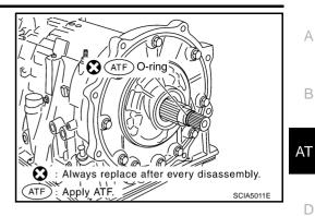
Remove tightening bolts for oil pump assembly and transmission case.
