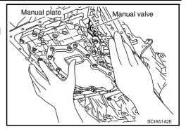
17. Remove A/T fluid temperature sensor 2 with bracket from control valve with TCM.
