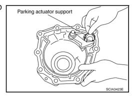
73. Remove parking pawl (with return spring) and pawl shaft from rear extension (2WD models) or adapter case (AWD models).
