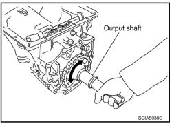
33. Install bearing race to output shaft.
