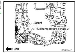
g. Install control valve with TCM in transmission case.
