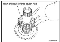
a. Remove needle bearing from high and low reverse clutch hub.
