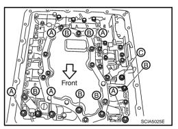
i. Tighten bolt 1, 2 and 3 temporarily to prevent dislocation. After that tighten them in order (1  $\rightarrow$  2  $\rightarrow$  3), and then tighten other bolts to the specified torque. Refer to <u>AT-274</u>, "Components".
