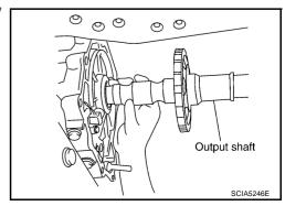
13. Remove parking gear from output shaft.
