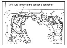
32. Straighten terminal clips to free terminal cord assembly and A/T fluid temperature sensor 2 harness.
