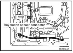
15. Straighten terminal clip to free revolution sensor harness.
