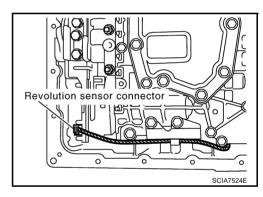
13. Securely fasten revolution sensor 2 harness with terminal clip.
