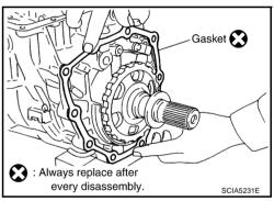
ii. Install adapter case assembly to transmission case.
