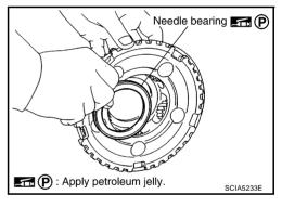
c. Install bearing race in front carrier assembly.
