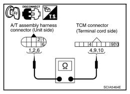
4. Check continuity between A/T assembly harness connector terminals and TCM connector terminals.
