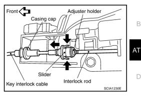
Remove holder (A) from key cylinder (1) and remove key interlock cable (2).
