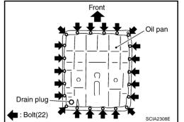
Tighten oil pan mounting bolts to the specified torque in numerical order shown in the figure after temporarily tightening them. Refer to AT-274, "Components".
