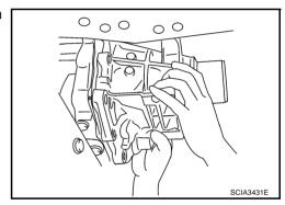
11. Remove bearing race from output shaft.
