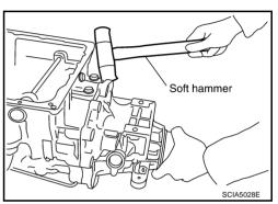
iii. Remove rear extension assembly from transmission case. (With needle bearing.)
