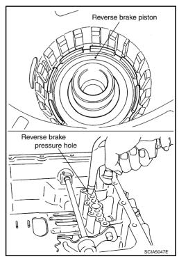
59. Remove D-rings from reverse brake piston.
