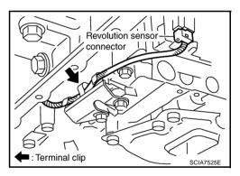
4. Apply recommended sealant (Genuine Anaerobic Liquid Gasket or equivalent. Refer to <u>GI-48</u>, "<u>Recommended Chemical Products and Sealants</u>" .) to rear extension assembly as shown in the figure.
