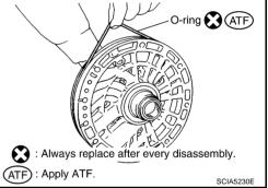
2. Install O-ring to oil pump housing.
