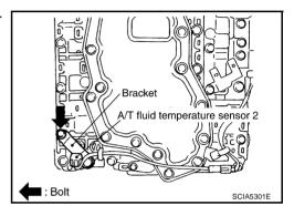
18. Remove bracket from A/T fluid temperature sensor 2.
