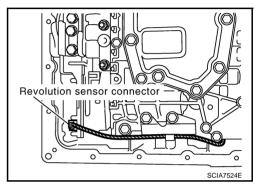
13. Securely fasten revolution sensor harness with terminal clip.
