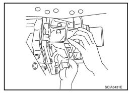
12. Tighten rear extension assembly mounting bolts to specified torque. Refer to <u>AT-251, "COMPONENTS"</u>.
