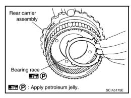
21. Remove needle bearing from rear carrier assembly.
