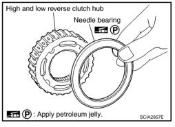
6. Install high and low reverse clutch hub to mid sun gear assembly.
