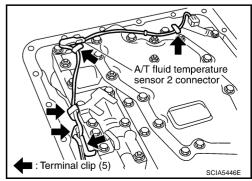
33. Disconnect revolution sensor connector.
