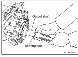
12. Remove output shaft from transmission case by rotating left/ right.
