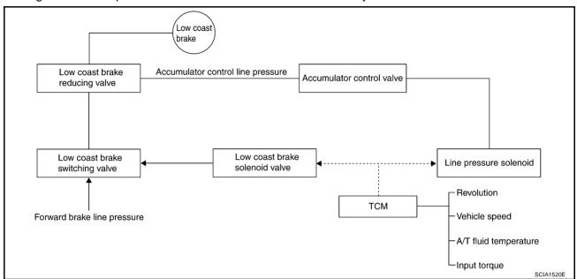
The operation of the low coast brake solenoid switches the low coast brake switching valve and controls
