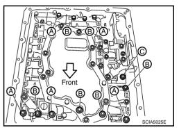
36. Remove control valve with TCM from transmission case.
