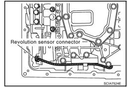
Securely fasten revolution sensor harness with clip.
