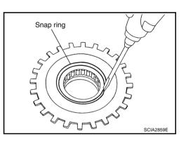
b. Remove 1st one-way clutch from rear sun gear.
