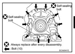
ii. Tap rear extension assembly with soft hammer.
