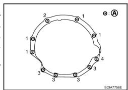
Align the positions of tightening bolts for drive plate with those of the torque converter, and temporarily tighten the bolts. Then, tighten the bolts with the specified torque. Refer to <u>AT-269</u>, <u>"COMPONENTS (FOR VQ35DE)"</u> or <u>AT-270</u>, <u>"COMPONENTS (FOR VK45DE)"</u>.
