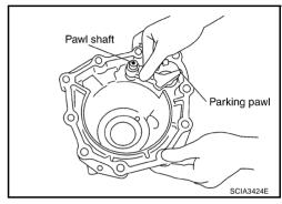
28. Install parking actuator support to rear extension (2WD models) or adapter case (AWD models).
