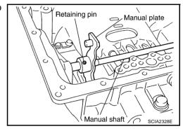
61. Remove manual shaft retaining pin with pair of nippers.
