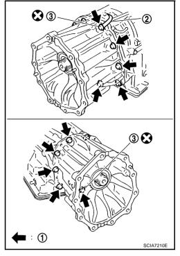
ii. Tap adapter case assembly with soft hammer.
