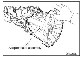
Tighten adapter case assembly mounting bolts (1) to specified torque. [With bracket (2) .] Refer to AT-274, "Components" .
