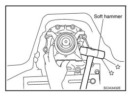
13. Remove rear extension assembly from transmission case. (With needle bearing.)
