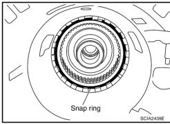
22. Measure clearance between retaining plate and snap ring. If not within specified clearance, select proper retaining plate. Refer to "Parts Information" for retaining plate.
