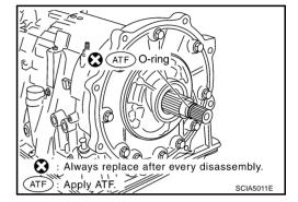
7. Install converter housing to transmission case, and then tighten converter housing mounting bolts to the specified torque. Refer to AT-274, "Components".
