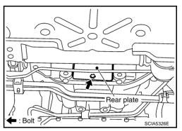
15. Turn crankshaft, and remove the four tightening bolts for drive plate and torque converter.
