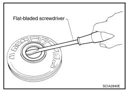
3. Remove O-ring from oil pump housing.
