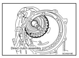
25. Remove needle bearing from drum support.
