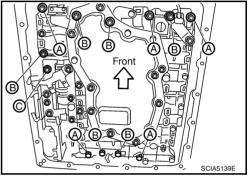
9. Tighten bolt 1, 2 and 3 temporarily to prevent dislocation. After that tighten them in order (1  $\rightarrow$  2  $\rightarrow$  3), and then tighten other bolts to the specified torque. Refer to <u>AT-239</u>, "COMPONENTS"
