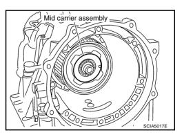
17. Remove mid carrier assembly from rear carrier assembly.
