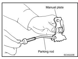
64. Remove manual shaft from transmission case.
