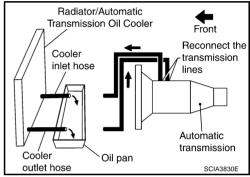
Insert the extension adapter hose of a can of Transmission Cooler Cleaner (Nissan P/N 999MP-AM006) into the cooler outlet hose.
