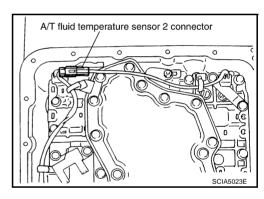
8. Straighten terminal clip to free A/T fluid temperature sensor 2 harness.
