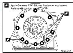
Tighten oil pump mounting bolts to specified torque. Refer to AT-274, "Components"
