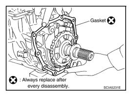
44. Remove bearing race from output shaft.
